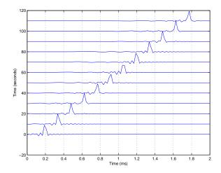
**Fig. 1:** Recorded Impulse Train with Clock Drift. A two-minute long recorded impulse train in the presence of clock drift.
