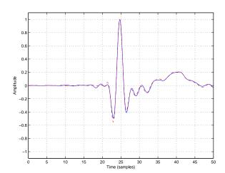
Fig. 7: Impulse Response with Compensation. Impulse response with drift compensation (dashed) using explicit clock drift estimation and windowed since interpolation plotted against a reference impulse response with no drift (solid).
