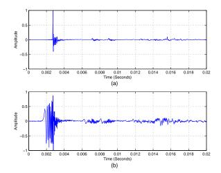
Fig. 2: (a) Room Impulse Response without Clock Drift. A reference room impulse response measured without clock drift using a single audio interface for playback and recording. (b) Room Impulse Response with Clock Drift. A room impulse response measured in the presence of clock drift using two unsynchronized audio interfaces for playback and recording.
