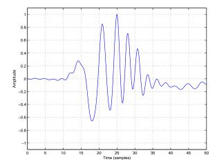
**Fig. 6:** Impulse Response Direct Path With Clock Drift. The direct path of an impulse response in the presence of clock drift used for comparison with Fig. 7 and Fig. 8.
