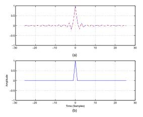
Fig. 3: (a) Impulse Responses Using Time-Reversal Mirror and Closed-Form Inverse Approaches. Impulse responses computed using inverse filters via time-reversal mirror (dashed dot) and closed-form (dashed) approaches showing roughly bandlimited inversion. (b) Impulse Response Using the Numerical Inversion Inverse Approach. An impulse response computed using an inverse filter created via numerical inversion showing an improved result.
