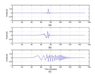
Fig. 5: (a) Reference Impulse Response. A reference impulse response without clock drift. (b) Impulse Response via Exponential Sine Sweep. An impulse response in the presence of clock drift computed using an exponential frequency trajectory sine sweep input. (c) Impulse Response via Linear Sine Sweep. An impulse response in the presence of clock drift computed using a linear frequency trajectory sine sweep input.
