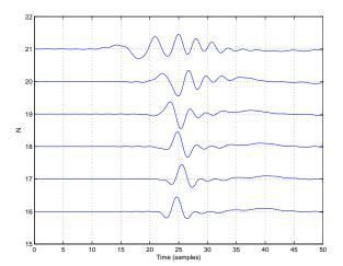
**Fig. 4:** Various Length Impulse Responses with Clock Drift. Impulse responses in the presence of clock drift computed using various length input sine sweeps.
