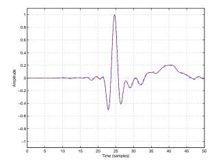
Fig. 8: Impulse Response with Compensation. Impulse response with drift compensation (dashed) using implicit clock drift estimation and compensation plotted against a reference impulse response with no drift (solid).
